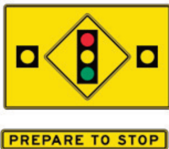
Figure 10-15: Advanced Warning Flashers and Sign
