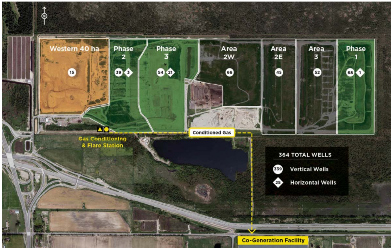
FIGURE 3 - LANDFILL GAS COLLECTION SYSTEM 2015
