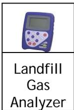
A LFG analyzer is a portable instrument that can measure methane concentrations from 0% to 100% by volume and LEL, and oxygen concentrations from 1% to greater than 21%. This instrument is not to be used as a personal gas detector but is used to measure concentrations of LFG in pipes and equipment.
