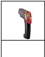
Infra-red thermometers shall be used from time to time to verify that surfaces have cooled sufficiently to allow for human contact. In particular, infra-red thermometers may be used to verify the temperature of flare stacks prior to working on or around the stack.
